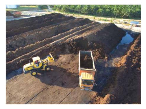
The POME collected from the mill is treated in open anaerobic ponds located on site. The organic material in wastewater is broken down by natural occurrences of anaerobic and aerobic bacteria. This process eliminates the need to add chemicals before the water is discharged and results in successful fish breeding at the final effluent pond. POME is utilised in two ways. It is either mixed with shredded EFB to make our compost or applied directly to estate via the furrow system.
